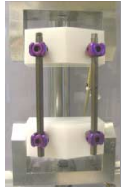
Fatigue test on spinal implant in a vertebrectomy construct
