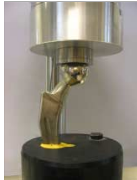
Fatigue test on femoral stem
