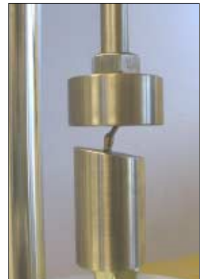
Fatigue test on dental implant
