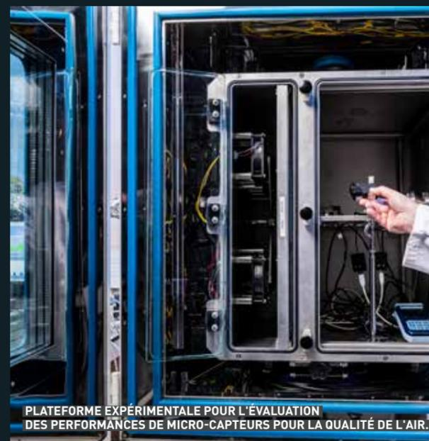
PLATEFORME EXPÉRIMENTALE POUR L'ÉVALUATION DES PERFORMANCES DE MICRO-CAPTEURS POUR LA QUALITÉ DE L'AIR.
