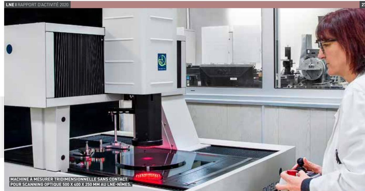
MACHINE À MESURER TRIDIMENSIONNELLE SANS CONTACT POUR SCANNING OPTIQUE 500 X 400 X 250 MM AU LNE-NÎMES.
