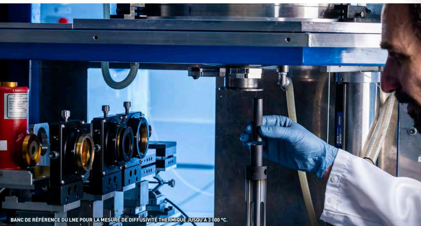
BANC DE RÉFÉRENCE DU LNE POUR LA MESURE DE DIFFUSIVITÉ THERMIQUE JUSQU'À 3 000 °C.
