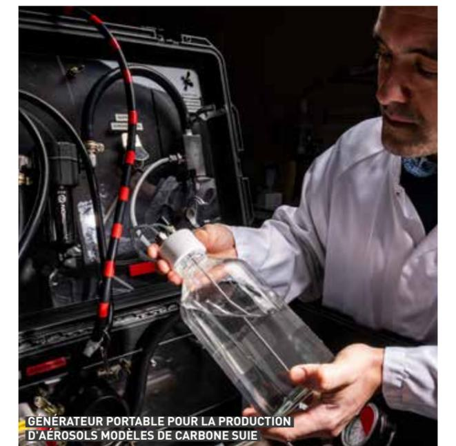
GÉNÉRATEUR PORTABLE POUR LA PRODUCTION D'AÉROSOLS MODÈLES DE CARBONE SUIE
