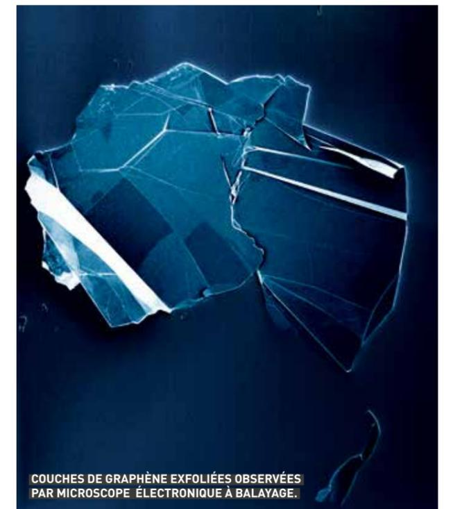
COUCHES DE GRAPHÈNE EXFOLIÉES OBSERVÉES PAR MICROSCOPE ÉLECTRONIQUE À BALAYAGE.
