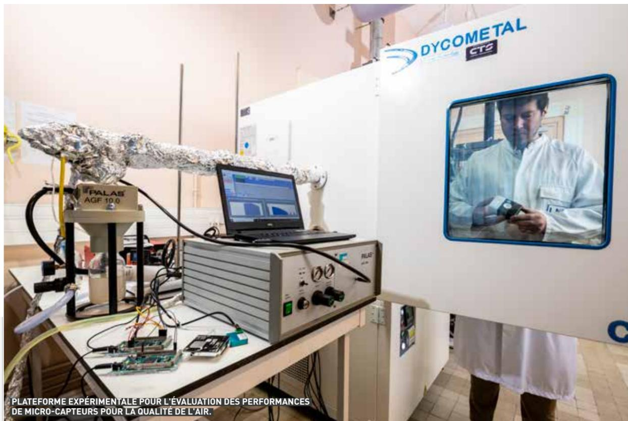
PLATEFORME EXPÉRIMENTALE POUR L'ÉVALUATION DES PERFORMANCES DE MICRO-CAPTEURS POUR LA QUALITÉ DE L'AIR.
