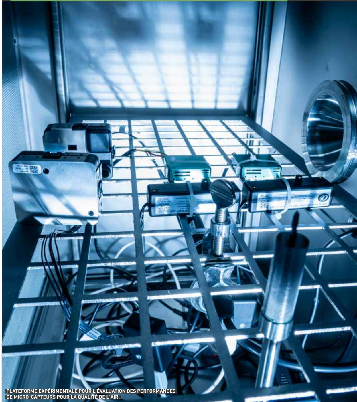
PLATEFORME EXPÉRIMENTALE POUR L'ÉVALUATION DES PERFORMANCES DE MICRO-CAPTEURS POUR LA QUALITÉ DE L'AIR.
