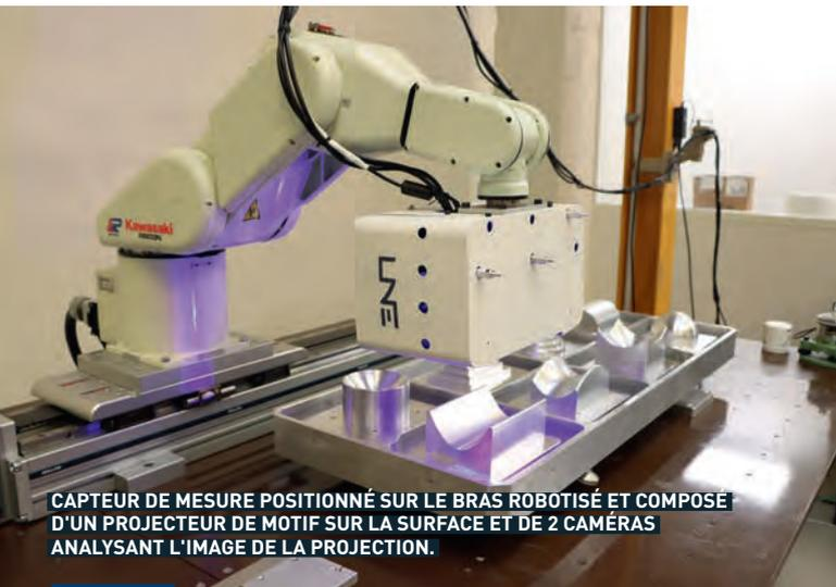
**CAPTEUR DE MESURE POSITIONNÉ SUR LE BRAS ROBOTISÉ ET COMPOSÉ D'UN PROJECTEUR DE MOTIF SUR LA SURFACE ET DE 2 CAMÉRAS ANALYSANT L'IMAGE DE LA PROJECTION.**
