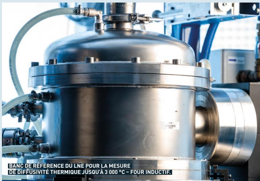
**BANC DE RÉFÉRENCE DU LNE POUR LA MESURE DE DIFFUSIVITÉ THERMIQUE JUSQU'À 3 000 °C – FOUR INDUCTIF.**
