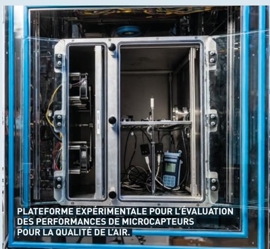
PLATEFORME EXPÉRIMENTALE POUR L'ÉVALUATION DES PERFORMANCES DE MICROCAPTEURS POUR LA QUALITÉ DE L'AIR.
