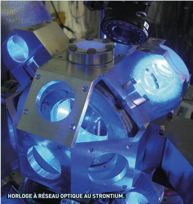
HORLOGE À RÉSEAU OPTIQUE AU STRONTIUM.
