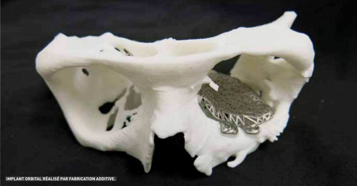
IMPLANT ORBITAL RÉALISÉ PAR FABRICATION ADDITIVE.
