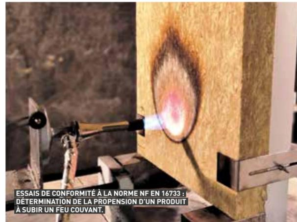
ESSAIS DE CONFORMITÉ À LA NORME NF EN 16733 : DÉTERMINATION DE LA PROPENSION D'UN PRODUIT À SUBIR UN FEU COUVANT.
