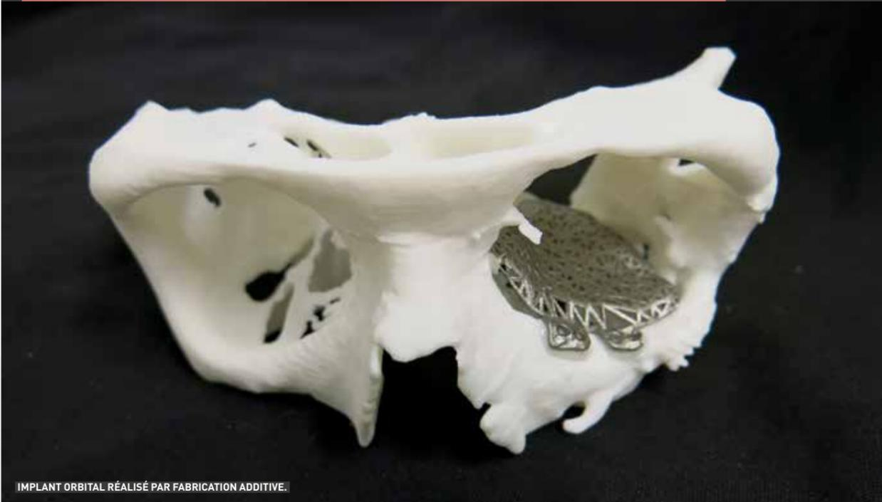
IMPLANT ORBITAL RÉALISÉ PAR FABRICATION ADDITIVE.
