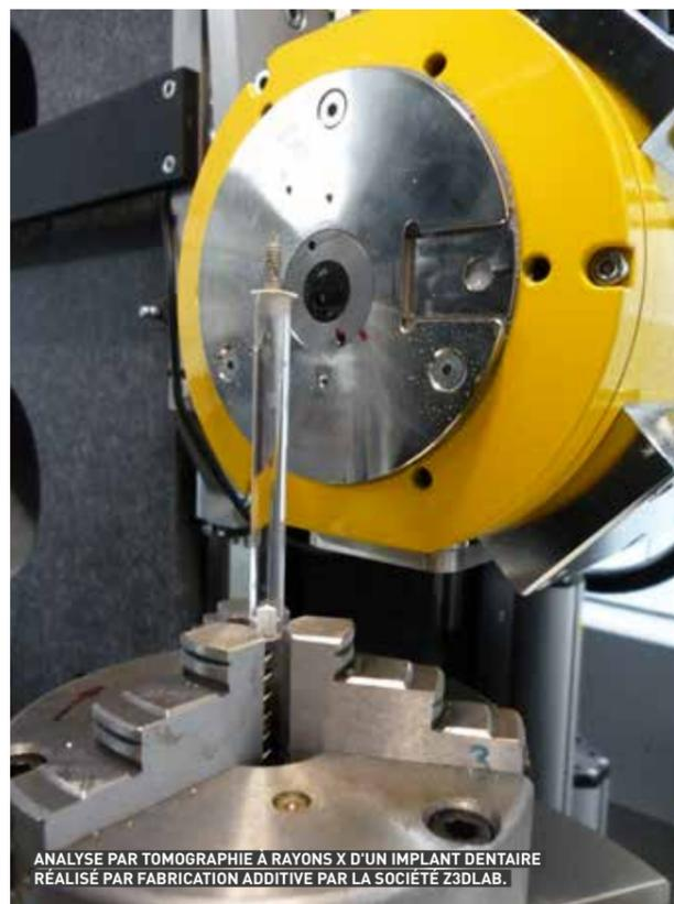
ANALYSE PAR TOMOGRAPHIE À RAYONS X D'UN IMPLANT DENTAIRE
