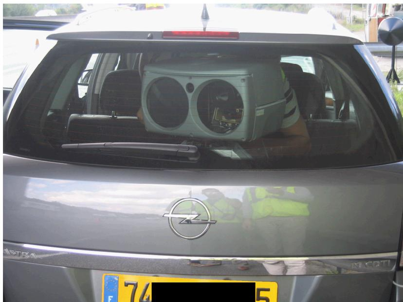
**EXEMPLE D'INSTALLATION DANS UN VEHICULE A L'ARRET DU MESTA 1x00**
