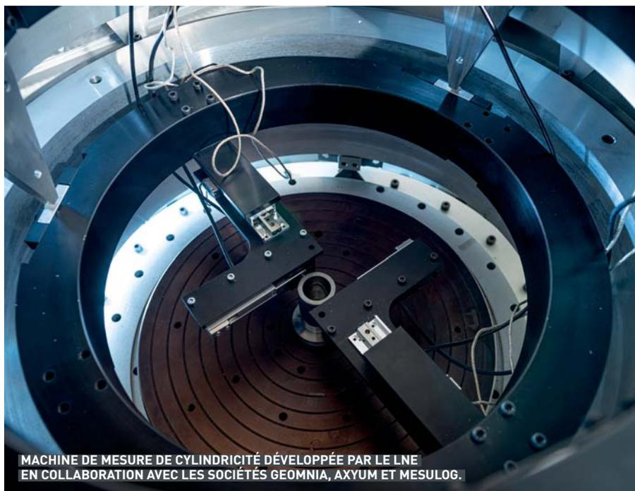
MACHINE DE MESURE DE CYLINDRICITÉ DÉVELOPPÉE PAR LE LNE EN COLLABORATION AVEC LES SOCIÉTÉS GEOMNIA, AXIUM ET MESULOG.
